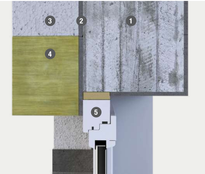
INSTALLATION OF FIRE PROTECTION WITH A WINDOW ON THE EDGE OF THE LOAD BEARING STRUCTURE
