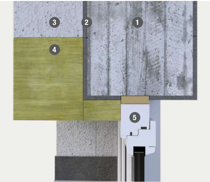
INSTALLATION OF FIRE PROTECTION WITH A WINDOW IN THE CENTRE OF THE BEARING STRUCTURE
